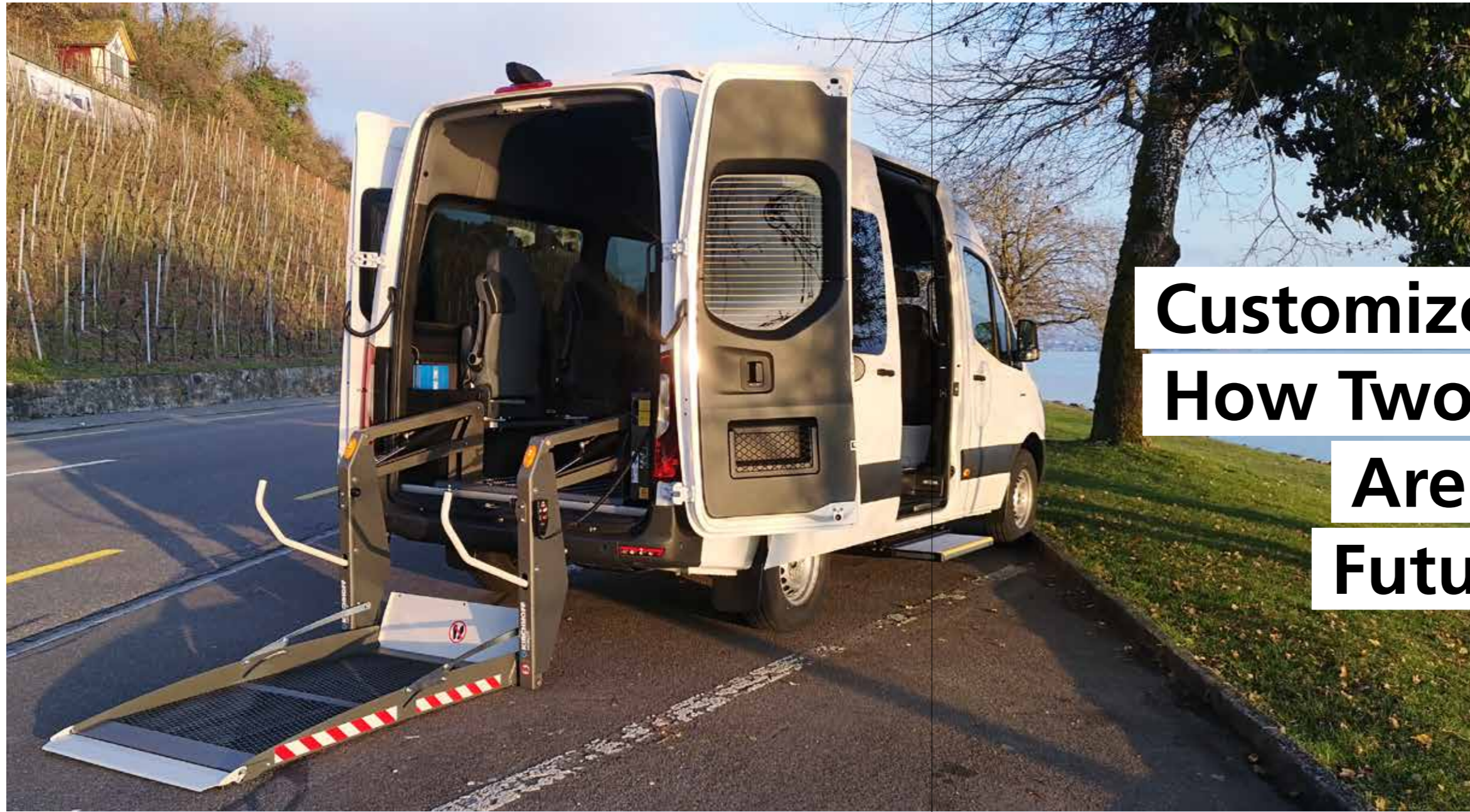
The Mercedes-Benz eSprinter was converted by KIRCHHOFF Mobility into a BTW 9-seater for passenger and accessible transport (up to 4 wheelchair users).
