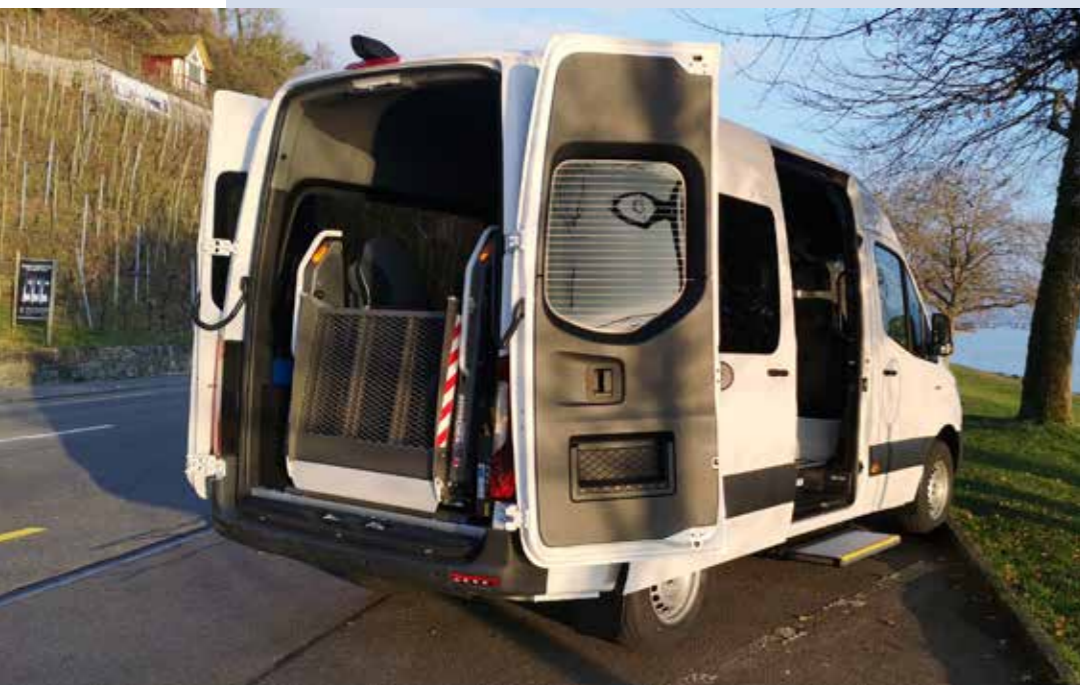
The Mercedes-Benz eSprinter was converted by KIRCHHOFF Mobility into a BTW 9-seater for passenger and accessible transport (up to 4 wheelchair users).
