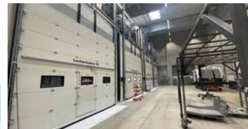
Two preparation and two painting cabins are part of the new paint line. Blasted components are painted in the customer's desired color in four process steps (body painting as standard). Heat recovery is achieved by means of high-efficiency heat wheels.
